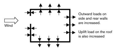
If more air is allowed to pass through the rear and side walls, the building is depressurized and air from within is sucked out of the building. This suction pressure pulls the side
