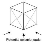
As the direction of these lateral loads cannot be predicted, the shear strength must be considered for loads from any direction. Therefore all walls should be designed to resist lateral loads.
