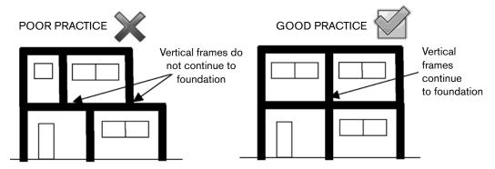
Vertical framing that does not continue to the foundation is a critical weak spot.
