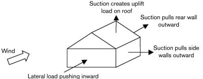
These loads may be increased or decreased based on the pressure within the building. If more air is allowed to pass through the wall facing the wind (via broken windows, severed doors, and any existing openings) the air pressure within the building will increase. This increase in air pressure inside the building will force the walls outwards. This will increase the outward pressure already exerted on the side and rear walls and roof.
