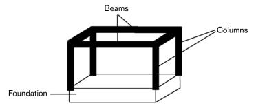
As the columns and beams joined together must resist the lateral loads, their joints must be made substantially rigid so as to maintain the box-like form. These joints are a critical point and must be securely fastened such that the joint is stronger than the structural members. Diagonal bracing can further increase the structure's lateral resistance
