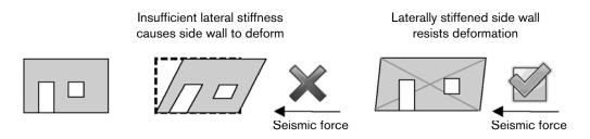
If this stiffness is insufficient relative to the load, the building will sustain damage and possibly collapse.
