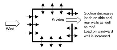
walls, rear wall and roof inward. This inward force counteracts the suction force of the wind outside the building. Therefore the load on the side and rear walls and on the roof are diminished.
