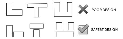
E10. Design building to be vertically regular with respect to lateral stiffness and weight distribution.
