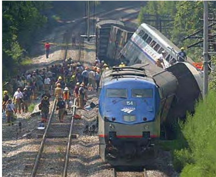
Figure 22: Trains can derail due to extreme heat warping railroad tracks.
