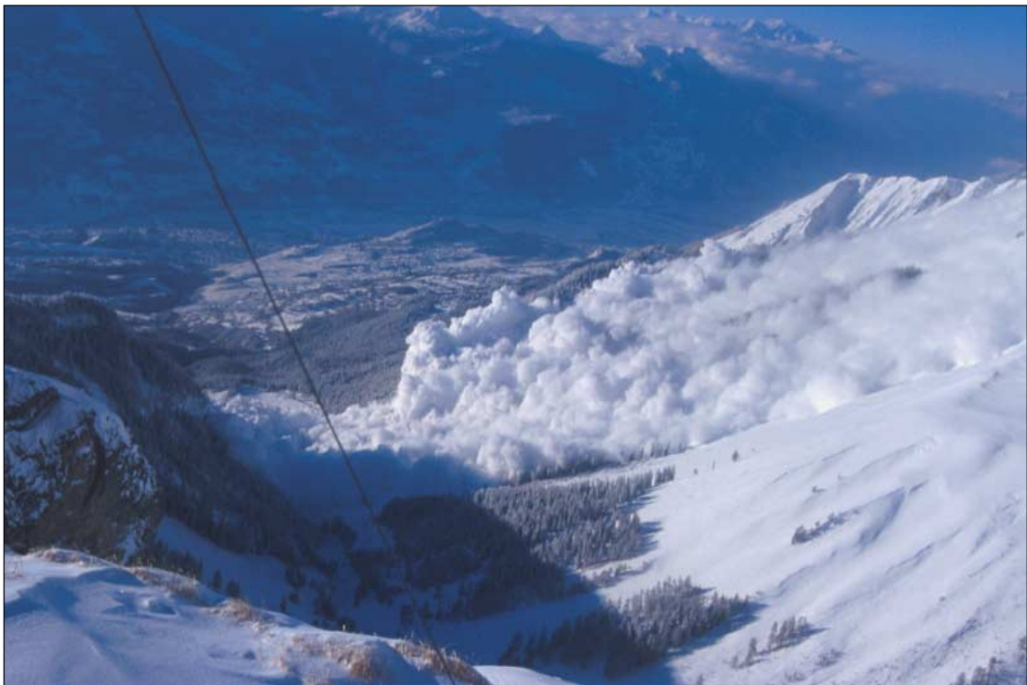
Figure 4.7 Artificially triggered powder snow avalanche in February 1999 at the avalanche test site Vallée de la Sionne of the Swiss federal Institute for Snow and Avalanche Research (SLF), Davos
