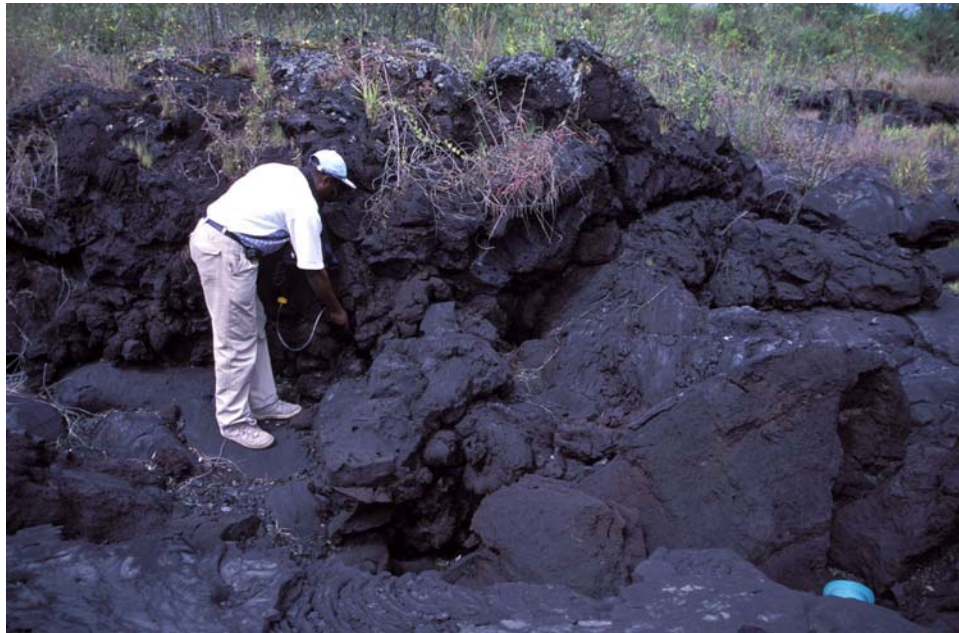
Fig.9. Measuring carbon dioxide concentrations in air: the gas flows out of the ground fissure at this mazuku , where deaths have occurred in the past.
