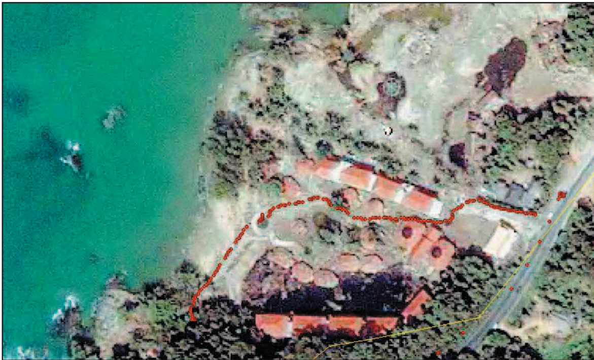
Figure 5. An example of a survey location in a heavily damaged Khao Lak resort in Phang Nga where foot based deployment was undertaken. The survey route is depicted by GPS points (red dots) along which georeferenced video and photographs were collected.
