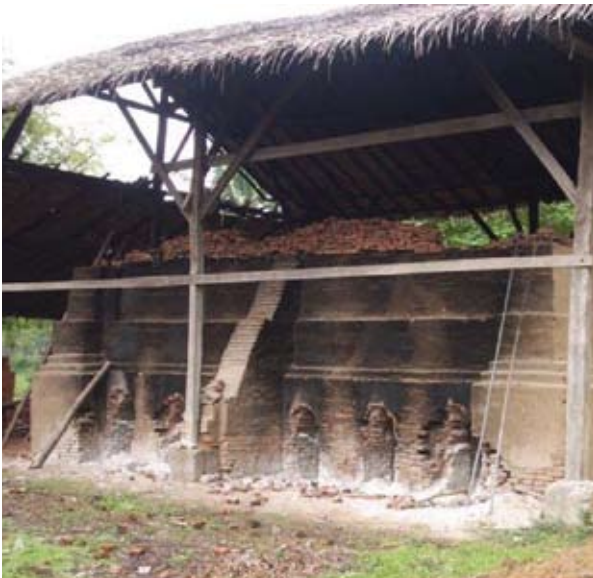
Figure 13: Typical brick kiln with low efficiency in the use of fuel wood (Photo: Niclas Svenningsen).
