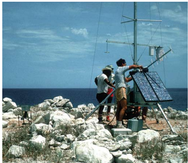
Portable, automated weather station on the Baja Peninsula of Mexico
