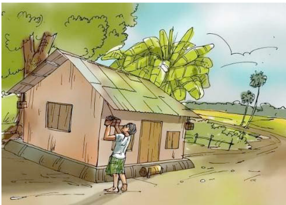
Hanging weights from the four corners of the roof during cyclone season
