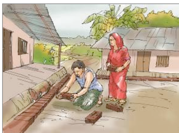
Laying bricks in a row to prevent damage to plinth area from rain water falling from roof
