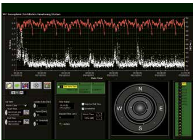
Observation of the ionospheric scintillation events at the JRC's Jicamarca monitoring station in the calendar week number 40 of 2012, showing clearly peaks of high scintillation activity occurring after the sunset typically within the period 00:00-04:00 UTC, which were particularly intense on October 1st 2012.
