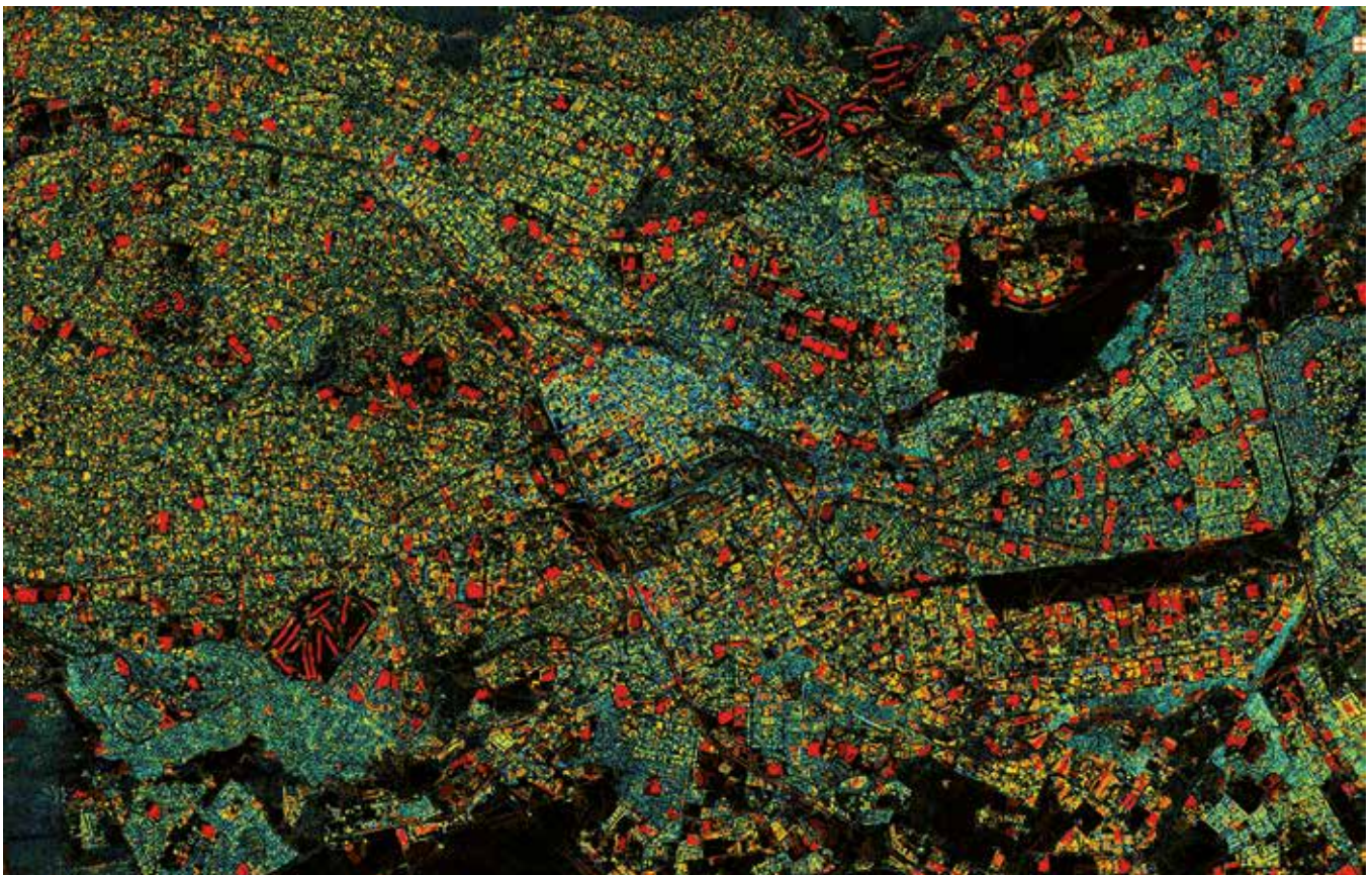
Information from the Global Human Settlements Layer (GHSL) over London: black areas are classified as not built-up, while different colours point to automatically detected built-up structures with different morphological characteristics.
