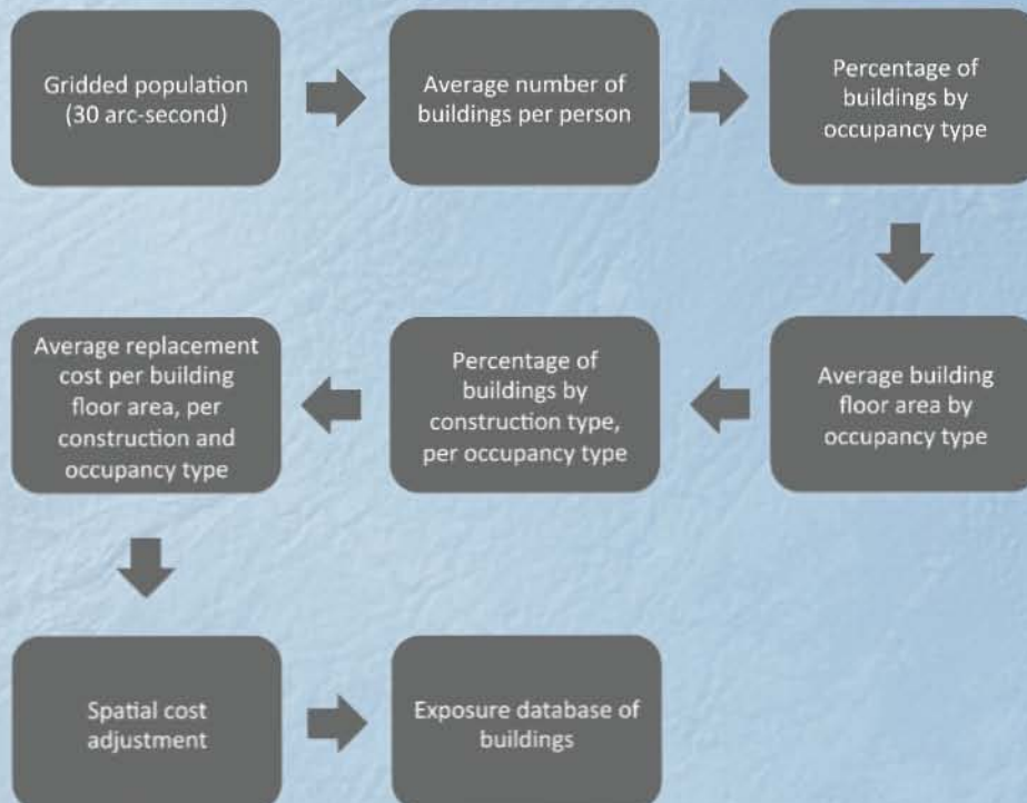
Figure A1. Schematic diagram illustrating the methodology used to develop the SWIO-RAFI exposure data
