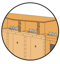
A35 Framing Angles Connect the Cripple Wall to the Floor System
