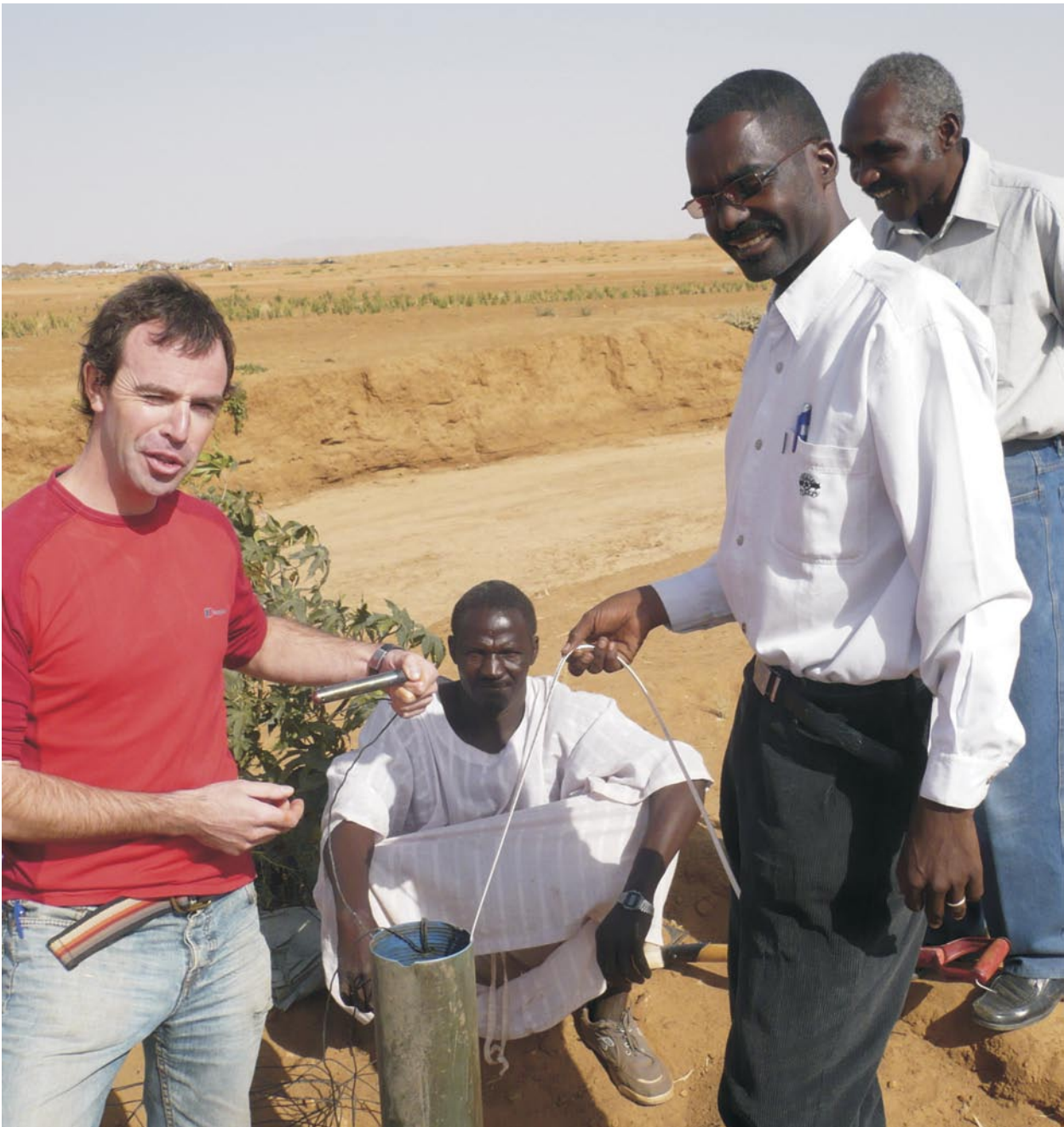
Figure 9. A logger (left) which records water levels and remains in the well. A dipper is being held down the well (right).
