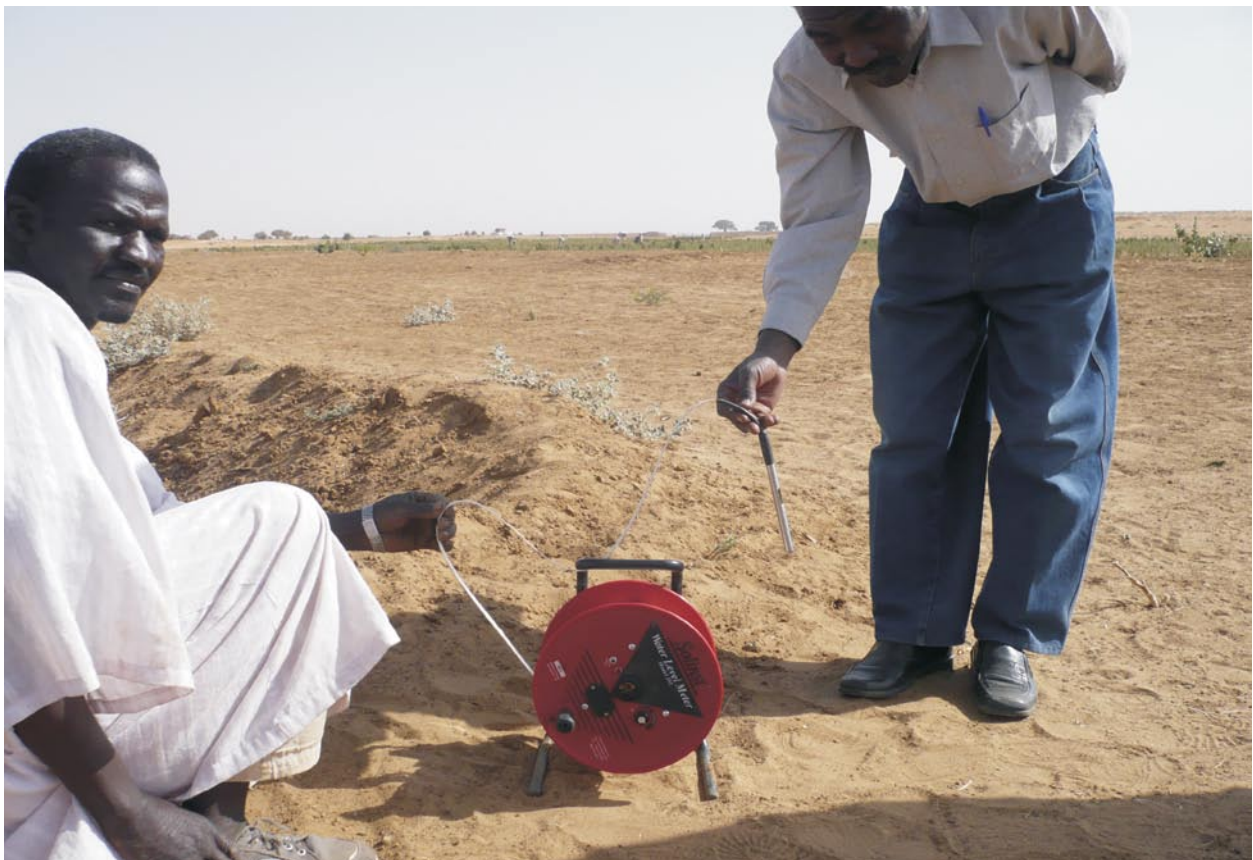
Figure 8. A “dipper” for manual measurement of water in a well. The sensor is on the end of a tape dropped down the well for a manual reading to water depth.
