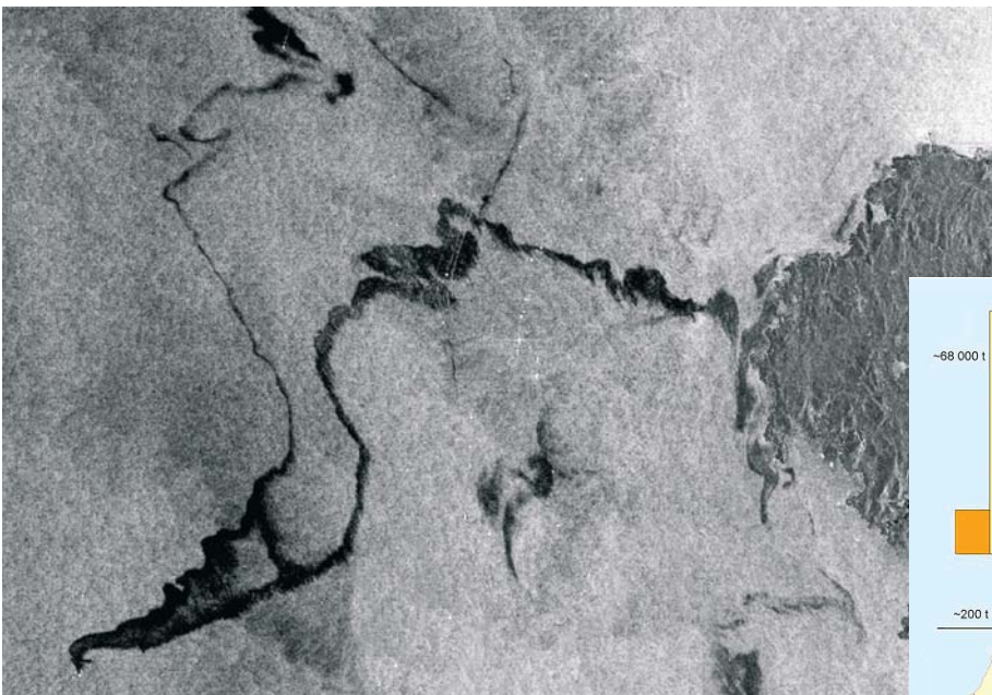
Oil slicks from the stranded tanker ‘Prestige’ as seen by Envisat’s ASAR instrument on 20 November 2002, and the total amounts of oil cleaned up on land and at sea in France, Spain and Portugal
