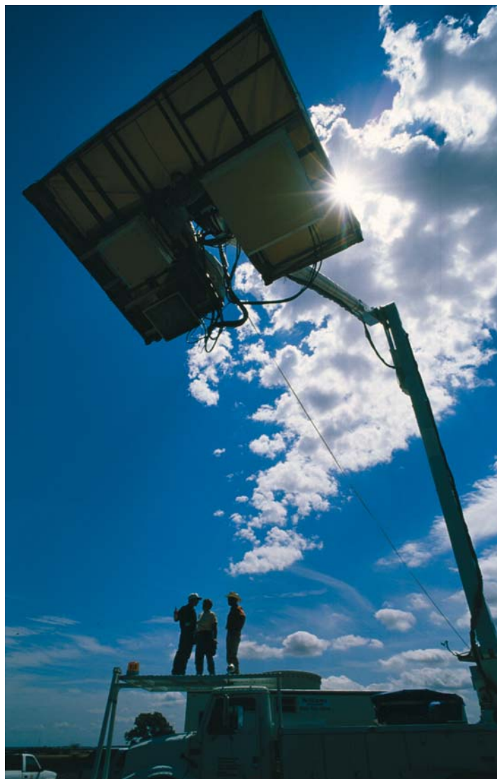
Boom-mounted microwave sounders mounted on a truck can quickly measure soil moisture
