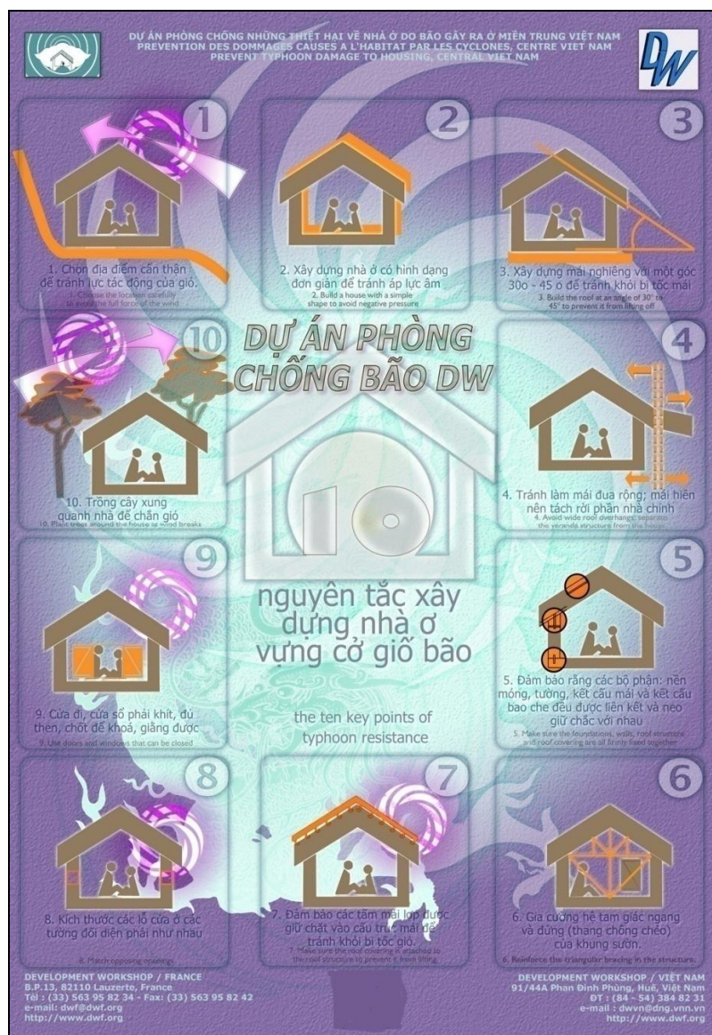
10 key points of typhoon resistant construction: generic principles that apply to all types of housing using local resources
