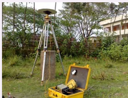
Setting coordinates for reference points in images using GPS technology
