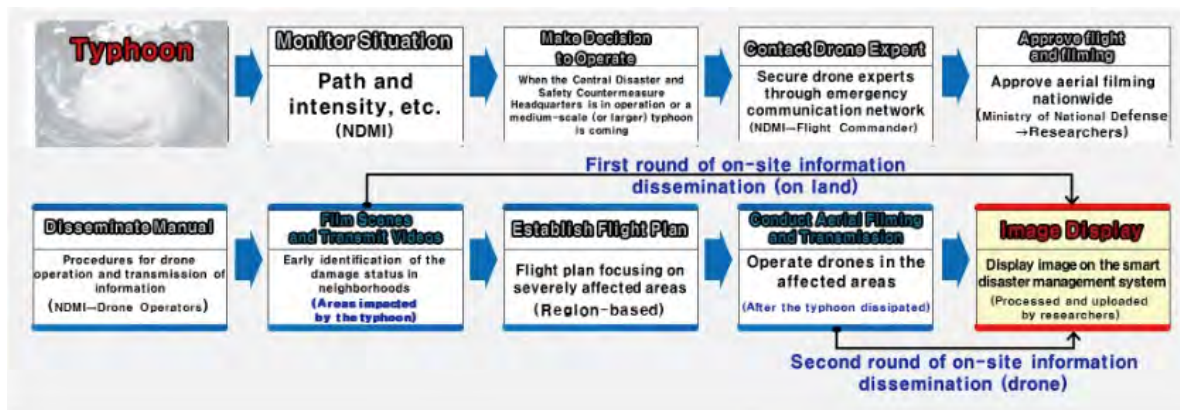
Figure 4. Emergency Drone Operation System for Typhoon Response (Source: National Disaster Management Research Institute)
