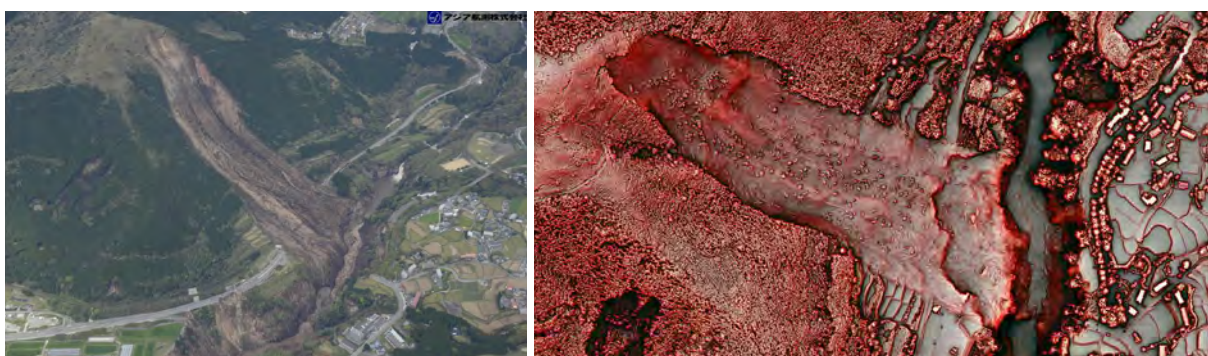
Figure 3. The Aso landslide was triggered by the Kumamoto Earthquake, April 16, 2016. a) Aerial photograph was taken after a few hours later the earthquake occurred; b) RRIM of the Aso landslide using Airborne Lidar data taken on April 16.
