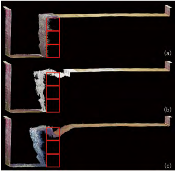
Figure 4. Results of 3D Measurements. (a) Before shake test. (b) After shaking at 203 Gals. (c) Residual deformation after final shake test
