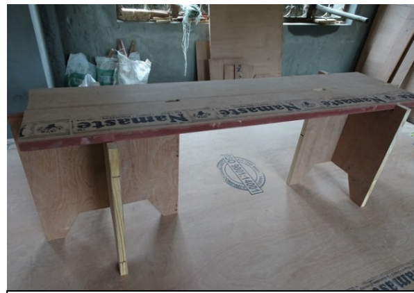
The parts are assembled to make the bench and does not require nails.
