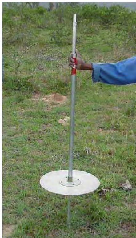
Figure 12.4. Disc Pasture Meter developed by Bransby & Tainton (1977) and used to estimate the grass fuel load for prescribed burning in African grasslands and savannas.
