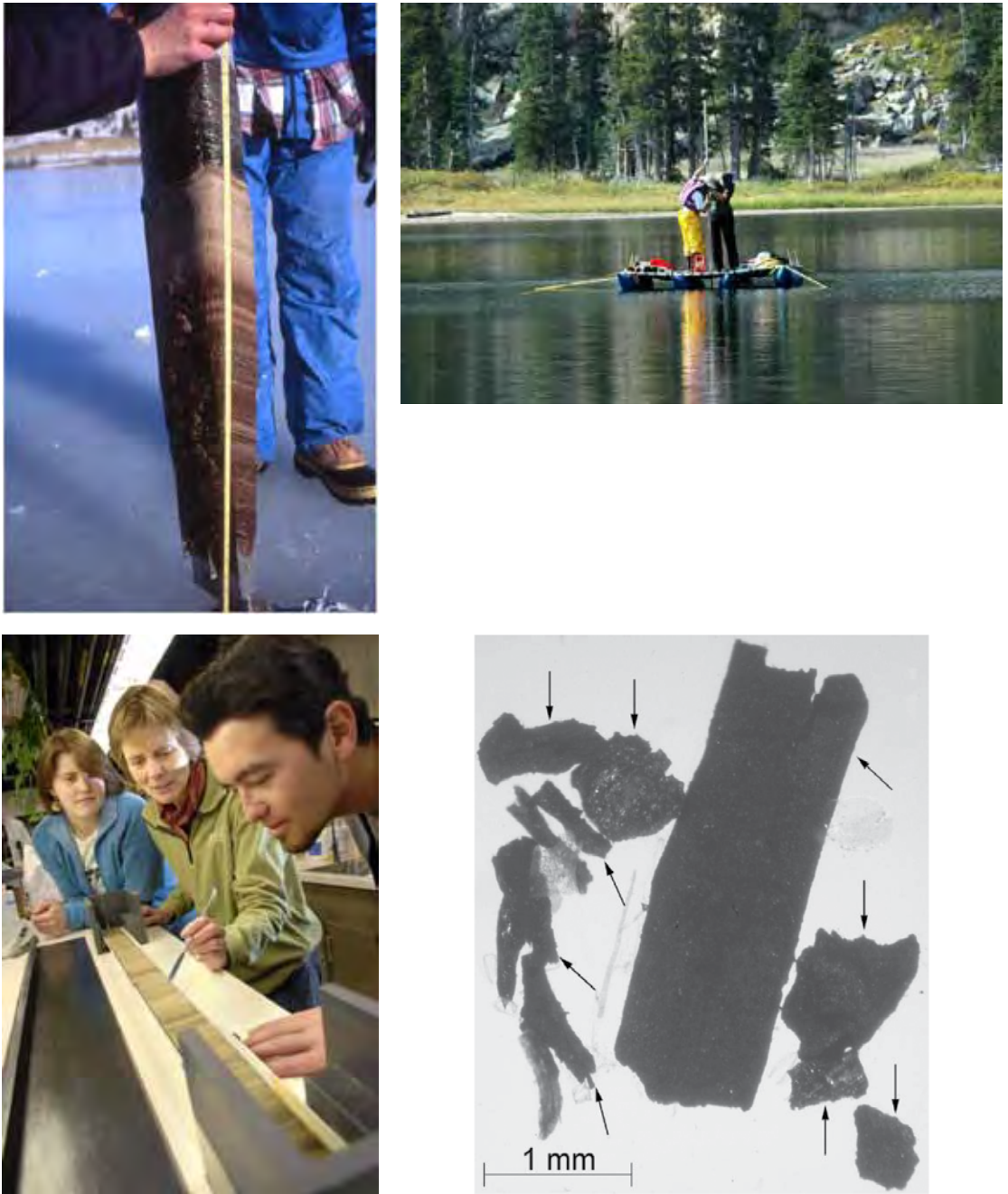
Figure 3.5. In high-resolution charcoal analysis sediment cores of lakes are recovered using various coring devices. Cores are split, described, and subsampled in the lab and the large particles of charcoal are quantified from continuous core samples (photo credits top left, clockwise: C. Whitlock, C. Adams, T. Minckley, and K. Gorham).
